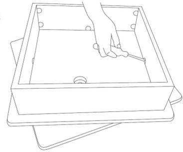
**NOTE:** If you do not want the spinner base to rotate, install a screw through the bottom base panel into the top base panel, taking care not to puncture through the surface of the top base panel. This will stabilize the spinner component of the base unit.
