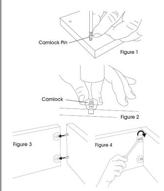
Using a #2 Phillips screwdriver, install the camlock pins into the pre-drilled holes in the (4) kick base boards. (See Figure 1)
