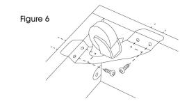
Position the casters onto each of the four corners of the kick base assembly. (See Figure 6)
